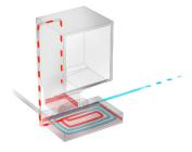
The effluent heat recovery system allows heat to be recovered from the hot water being drained to preheat cold water used for the next cycle. The system also greatly reduces the need to use cold water for drain cooling.
