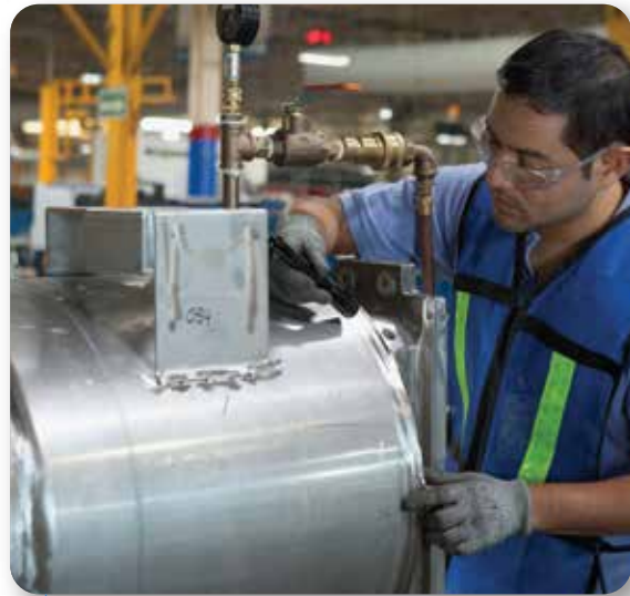
Each pressure vessel is individually inspected and hydro pressure tested.
