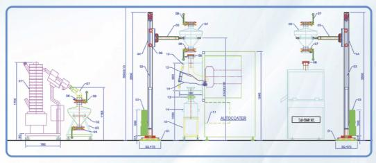
GroyneTech design GMP Hydraulic Lifter, Split Butter6ly Valve & Customize IPC for one step solution of "Close Loop Material Transfer System" with out affecting the PRODUCT, OPERATOR & ENVIRONMENT.
